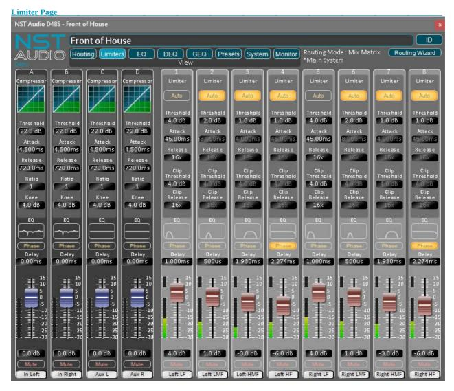
Pressing the Limiters button will show the output limiter parameters instead of the routing. The top parameters control the RMS limiter on each channel, and the lower parameters control the 'clip' or 'peak' limiters (Excluding D48 96kHz mode) giving a two-stage limiting system, which utilises our Predictive eXcursion Limiter (PXL) algorithm - designed to offer the best driver protection with the lowest distortion..
