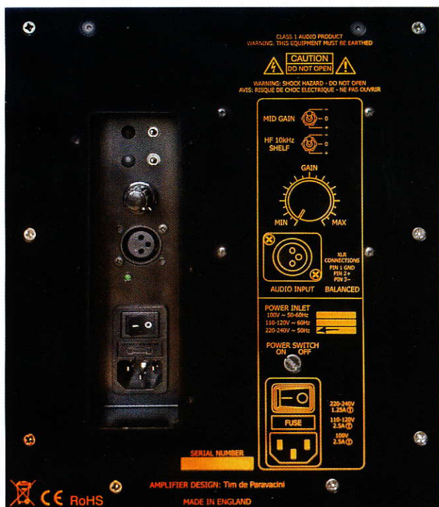
The Boulder's rear panel houses its mid-range and HF tuning controls, a gain pot, and the input XLR connector.
